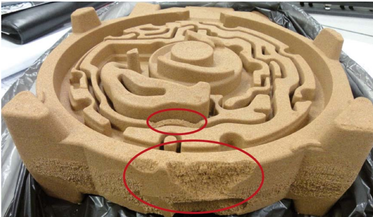
Figure 10: Defective core after curing. The marked areas shows the insufficiently cured regions of the core.
